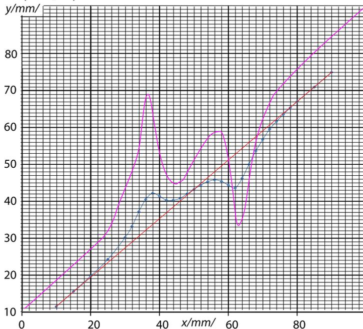
On this graph, the data of two different water levels are depicted; blue curve corresponds to a water depth of *ca* 2 mm (data given in the table above); the violet one — to 1 mm.
